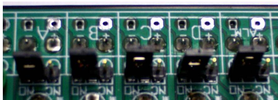
The relay output can be configured for normally open or normally closed contacts by using the jumper jacks located inside the unit located near the relays. The jumpers are marked “NC” for Normally Closed, and “NO” for Normally Open. Make sure that you have the jumper firmly connected to two pins, the center pin and one side pin to make the selection.
