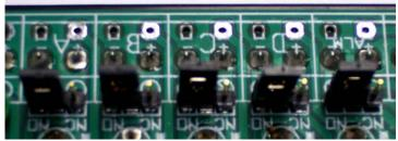
The relay output can be configured for normally open or normally closed contacts by using the jumper jacks located inside the unit located near the relays. The jumpers are marked "NC" for Normally Closed, and "NO" for Normally Open. Make sure that you have the jumper firmly connected to two pins, the center pin and one side pin to make the selection.
