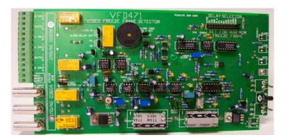
The VFD471 card fits into the RMS400  $\underline{\mathbf{R}}$  ack  $\underline{\mathbf{M}}$  ount  $\underline{\mathbf{S}}$  ystem, which is a 19" X 5 1/4" built-in power supply and Mainframe for use in a standard 19" rack. This rack mount will hold up to nine VFD471 cards. This lets you put nine independent video freeze frame switchers in three vertical rack spaces.
