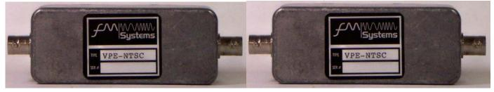
The VDE-NTSC is a video De-Emphasis Network for NTSC color video. It is used to offset triangular noise distribution created by FM transmission systems. FM fiber, Satellite and microwave transmission systems exhibit this kind of triangular noise pattern. This standard video De-Emphasis noise reduction technique requires "ROOFING". Roofing occurs when the video de-emphasis "signal curve" bottoms out, this prevents uncontrolled excessive high frequency roll-off.
