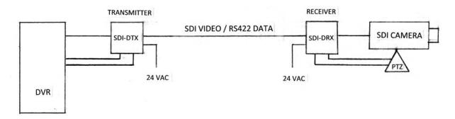
The equipment used to transmit and receive the RS422 signal is called SDI-DTX and SDI-DRX. There is a transmitter and a receiver used to provide an RS422 PTZ Data Link on any SDI coaxial cable. Use it to add (PTZ) control to any existing SDI video camera without running additional wires. The RS422 control signal shares the coaxial cable path in the opposite direction to control the camera without interfering with the SDI video image.
