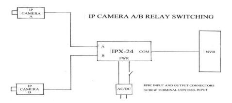
With analog camera signals these applications were accomplished with a simple video switch. But now with the new network cameras it is not as easy to do with just a single relay. To do the job the network switch must switch all 4 pairs of network wires and maintain the proper line impedance to reduce high frequency reflections that can reduce the quality of the IP network camera signal. It also must handle and switch the P.O.E. signal as well.
