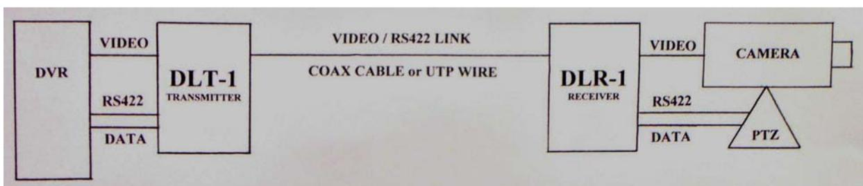
The equipment used to transmit and receive the RS422 signal is called DLT-1 and DLR-1, RS422 PTZ data link. There is a transmitter and a receiver used to provide an RS422 PTZ Data Link on any coaxial cable or UTP twisted pair wire video path. Use it to add (PTZ) control to any existing video camera without running additional wires. The RS422 control signal shares the video path in the opposite direction to control the camera without interfering with the video image.
