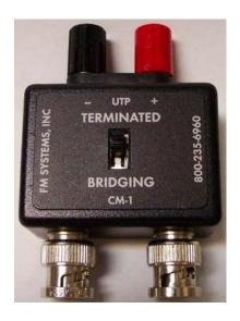
The CM-1 UTP is an adaptor that is used with the CM-1 CAMERA MASTER meter to measure the video levels on twisted pair wire installations. The adaptor conveniently mounts to the two BNC connectors on the top of the CM-1 CAMERA MASTER METER.
