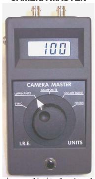
The Camera Master is a digital, hand-held, battery operated meter that measures five different characteristics of the video signal from a CCTV camera or other video sources, such as:
