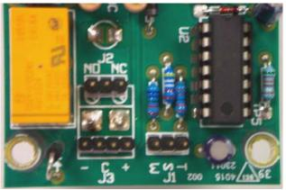
3. For Low Voltage output operation position one shunt onto J3 connecting the outermost two pins at the (+) mark and another shunt onto J3 at the other outermost two pins at the (-) mark. There should be two jumper shunts on this jack for supply voltage output. Then choose normally ON or normally OFF operation for the low voltage output and J2. For low voltage supply output this unit is available in two versions. The voltage output is supplied from the main 12 Volt power source.
