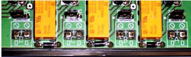
2. Locate the black jumper jacks next to the relays on the top of the PC Board. There are three gold pins under each jumper jack. Select (NO) for Normally Open. "NO" will cause the alarm contacts to close when the video fails. Or (NC) for Normally Closed. "NC" will cause the alarm contacts to open when the video fails. Make sure, that you place the jumper jack on two of the three pins for each of the 4 channels A-D. The top of the PC Board is marked with graphic to make programming easy.
