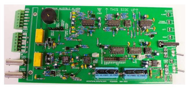
The AVI473 AUDIO Video Indicator provides two independent form C relay contact closures for loss of audio and video service. These contact closures can be used to operate an external program switch or remote maintenance alarm. The unit has an audible alarm sounder that can be separately field programmed for audio loss, stereo inversion, and video loss.
