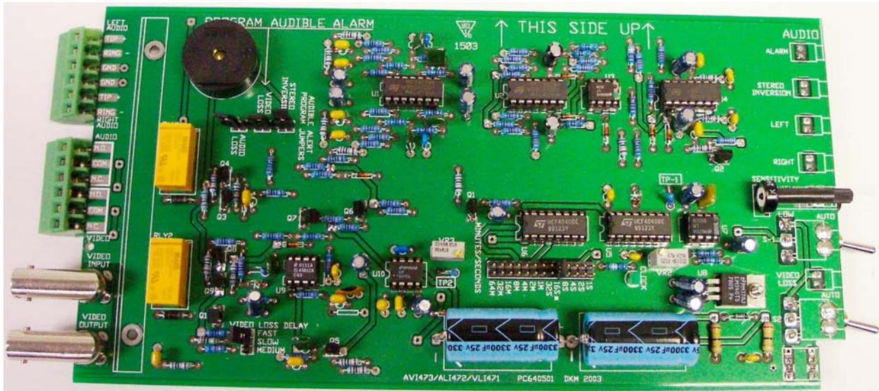
The **AVI473A AUDIO Loss Indicator** provides a form C relay contact closure for loss of Stereo audio service. This contact closure can be used to operate an external program switch or remote maintenance alarm. The unit has an audible alarm sounder that can be separately field programmed for audio loss on either channel or stereo inversion.
