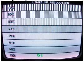
The VLTG-800 is a <u>V</u>ideo <u>L</u>ine <u>Test Generator</u> that creates a normal NTSC video picture with a test pattern consisting of 100, 200, 300, 400, 500, 600, 700, and 800 "Line" groups. Each of these groups of "Lines" is clearly identified so that you do not have to count the lines on the screen. Monitors may be tested "on the bench" by connecting the VLTG-800 directly to the Monitor under test.
