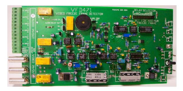
The VFD471 card fits into the RMS400 **R**ack **M**ount **S**ystem, which is a 19" X 5 1/4" built-in power supply and Mainframe for use in a standard 19" rack. This rack mount will hold up to nine VFD471 cards. This lets you put nine independent video freeze frame switchers in three vertical rack spaces.
