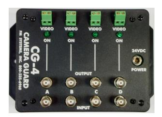
This unit can also be used to protect and alarm video monitors placed into public areas where theft of equipment is a concern. The CG-4 can be set to monitor the termination of the video signal so if the end of line equipment is disconnected from the video cable an alarm can be activated. A contact output will switch if the video cable is removed from the equipment.
