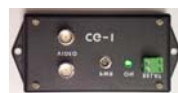
The CG-1 will handle 1 channel of HD-TVI video or an analog video signal.
